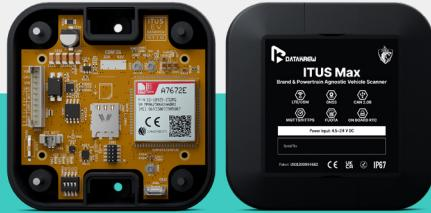
A rugged, brand and powertrain agnostic gateway that connects to any EV capturing high-resolution data (battery, driving, charging, telemetry) every 10 seconds
